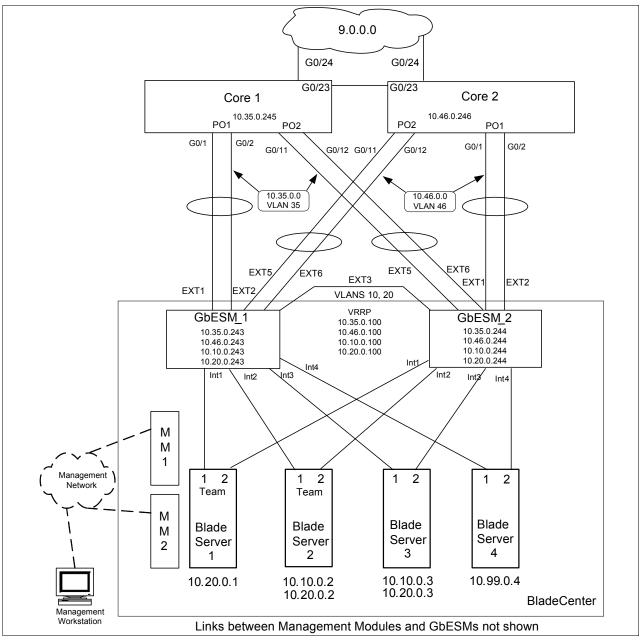
Figure 7-6 Layer 3 sample configuration (static routing, VRRP)
